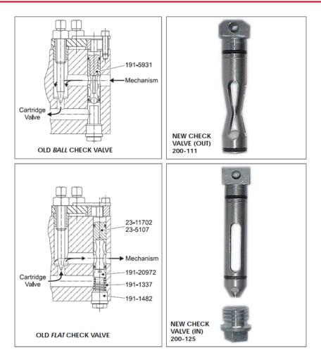
New generation Check Valves for the Electro-Pneumatic Valve Block
