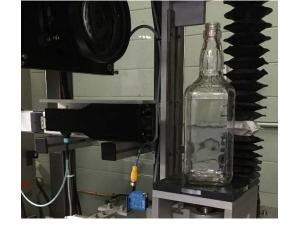
During the 360 degree rotation of the container the thickness sensor captures information to calculate the glass thickness at each location.
