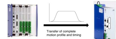
With **FlexIS 3** the controller uses the Motion Control technology and transfers the set point every 2-4 ms.
