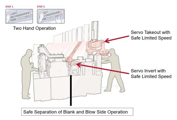
The new and safe Manual Mode introduces a safe Two Hand Operation for all Servo Mechanisms but also for the pneumatically moving mechanisms. A key element of the Manual Mode is the safe separation of the Blank and Blow side operation, which makes it possible to work safely inside the section on one side of the machine while the other side remains energized.
