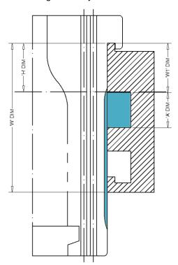
The total cooling air escape area on the fins needs to be carefully controlled and should not exceed 300mm<sup>2</sup>: the angular positioning needs to be maintained as shown on the sketch below.
