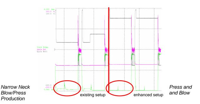
In Narrow Neck Press and Blow as well as Press and Blow the significant difference is the motion from the Down Position to Loading Position. The motion speed to the loading position and the precision of the loading position will be enhanced with the new setup. The Pressing and the Down Motion will remain unchanged.
